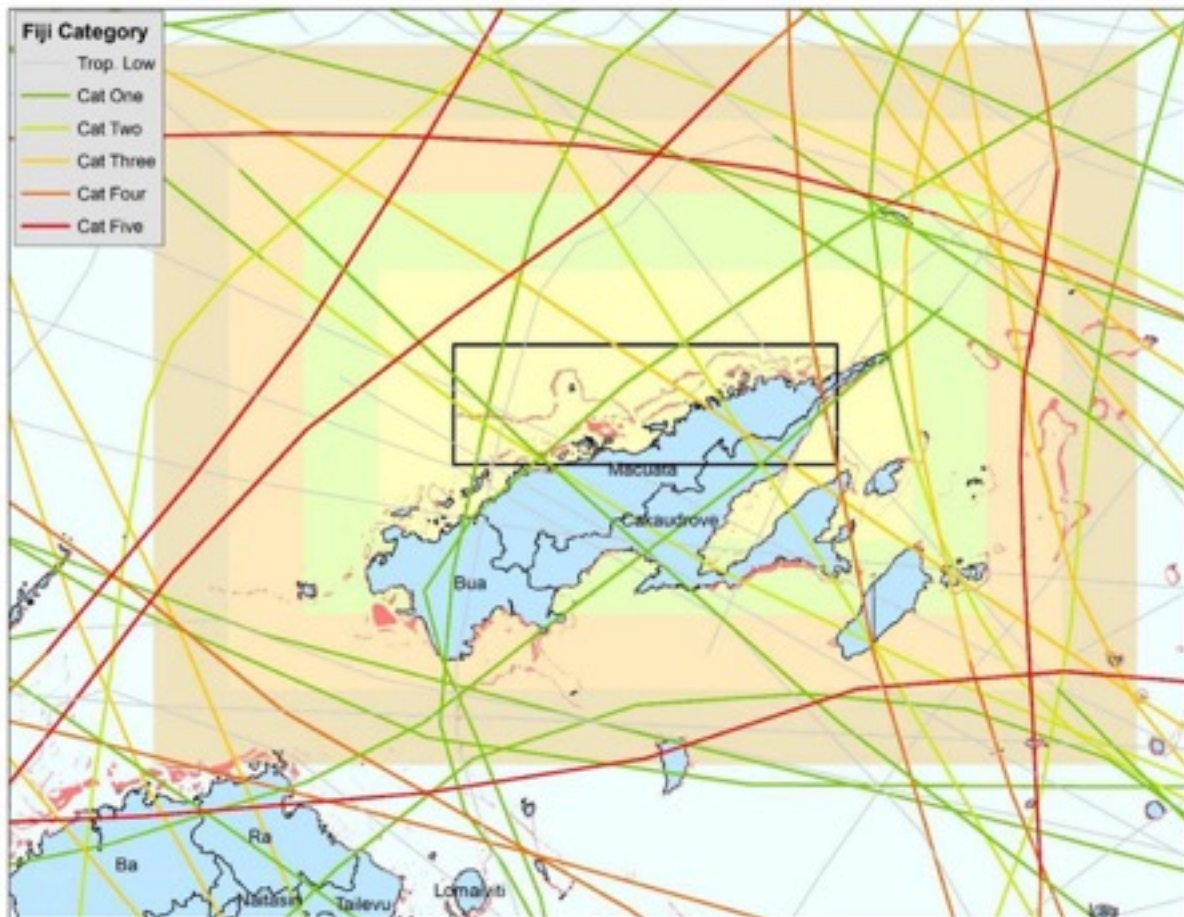
Figure 1.1 Testing historical cyclone activity within different buffer zones around the GSR offshore of Macuata province. The overall aim is to identify an area which captures storms which affect the reef but excludes storms which do not.
